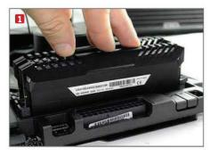
If necessary, push any unsecured clips properly into their notches to secure the memory. Do the same with any other modules. 1
