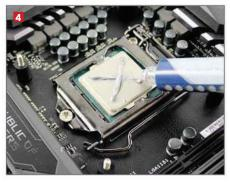
(TIM), also called thermal paste. Your cooler may come with a coating of TIM imprinted on the cooler's contact plate, ready for you to install; or you may be provided with a syringe to apply it yourself. 3 In the latter case, apply a thin cross shape from corner to corner on the heatspreader. 4The pressure from the mounting mechanism will spread the TIM across the rest of the CPU.
